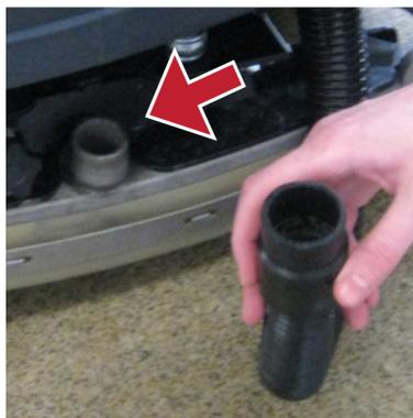
1 Check if the suction hose is correctly mounted and cleaned.
