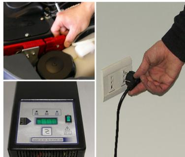
18. Charge the batteries: Connect the battery charger cable from the electrical main.
