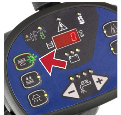
4 Check if the green switch Led is flashing. Wait until the light is steady.
