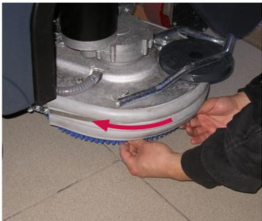
15. Remove the brush by turning as indicated with the figure and clean them.
