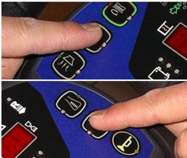
10. If necessary press the extra pressure function switch. If necessary press the mute function switch for reduce the noise.
