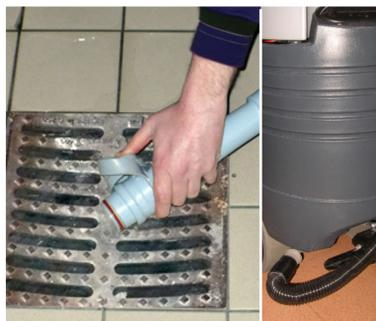
12. At the end of the work. Empty the recovery tank with the hose. Then empty the solution tank by opening the left drain tap and using the adapter and the vacuum system hose.
