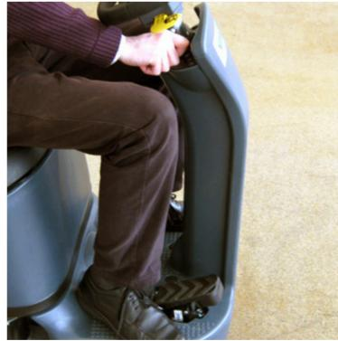
3 Turn the ignition key to "0", then try to start the machine without pressing the pedal speed.
