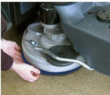
5. Place the brushes or the pad-holders under the deck. Use the appropriate brushes to clean the floor.
