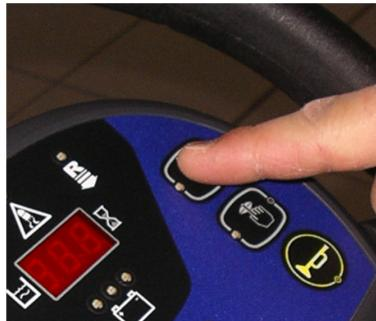
8. Press the detergent flow control switch. The number of display shows the detergent concentration level in the solution.
